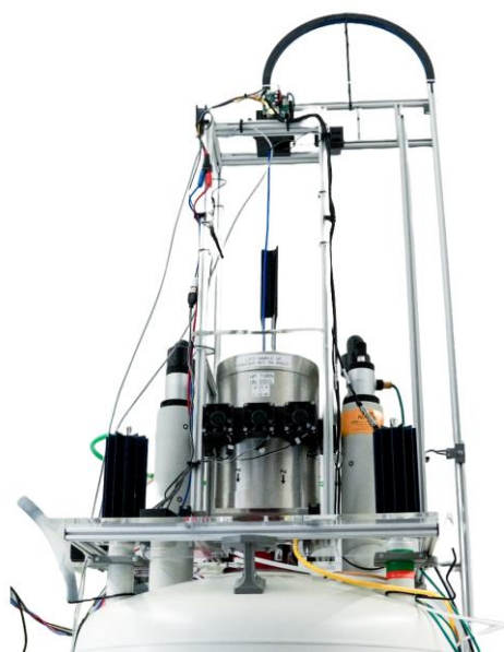
Fig. 1: A photo of the complete magnetic field cycling (MFC) device atop the spectrometer (NMR). The MFC enables the cycling of the NMR tubes from B0 magnetic field to the low magnetic field on top of the spectrometer. The MFC frame was mounted on a shelf positioned on top of the 400 MHz spectrometer.
