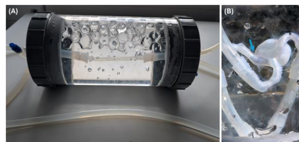
Fig. 1: (A) In-vitro flow phantom with embedded silicone tube (B) Image of the Derivo® flow diverter stent deployed inside an aneurysm phantom
